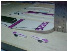
5. Glue wing to fuse using foam friendly CA. Be sure to align the wing to the fuselage properly before gluing.
