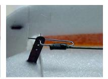
17. Adjust pushrod lengths until the surface are in their neutral positions when the actuators are center. To fix, put a small drop of Ambroid (or Duco, Sigment) glue on the pushrods to keep the "Z" bend and figure "4" from moving.
