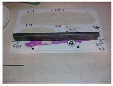
3. Add short piece of carbon fiber strip to front of radio box using a very thin coating of epoxy glue.
