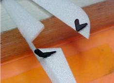
10. Hinge the elevator and rudder using short pieces of Blenderm.
