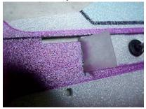
4. While the fuselage is drying, add the dihedral to the wings using foam friendly CA. Raise one wingtip 0.75 inch. Also, now is a good time to add the wheel pant doublers. Note a left and right pant needs to be made.
