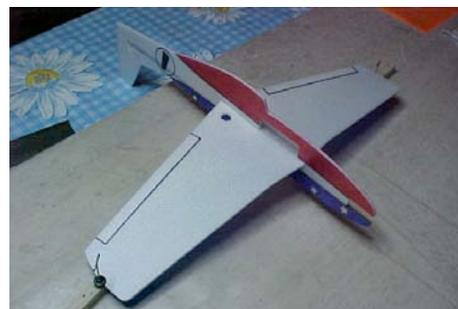
6. Prepare the horizontal tail by beveling the elevator leading edge. Add the Blenderm hinges. Add short piece of carbon fiber strip to center section of the elevator. (CA) Add the elevator horn.
