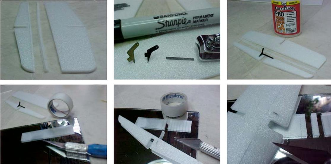
7. Glue horizontal stabilizer into the fuselage.
