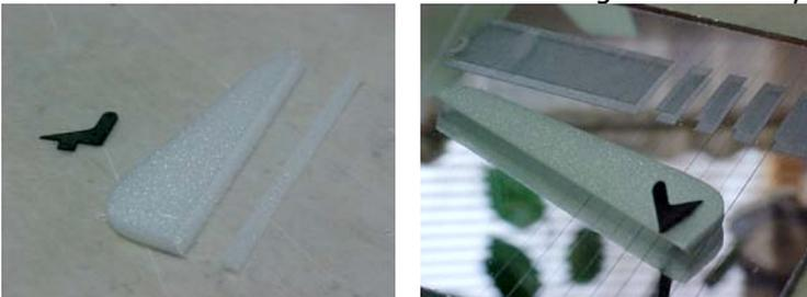
9. Hinge rudder using short pieces of Blenderm.
