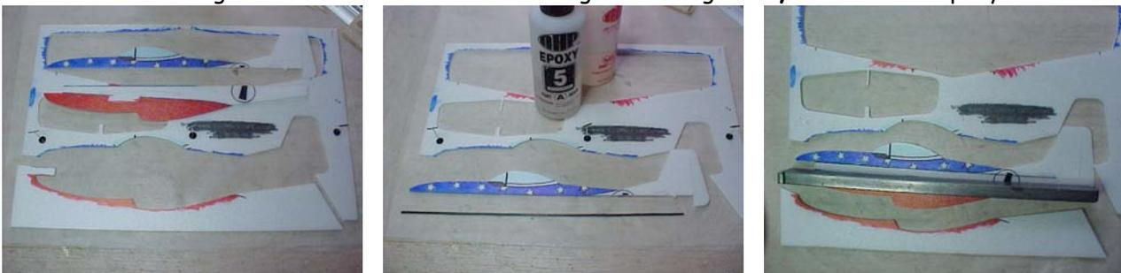
3. Add short piece of carbon fiber strip to front of radio box using a **very thin** coating of epoxy glue.
