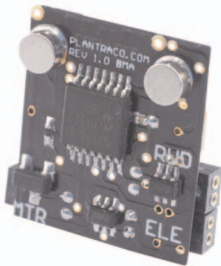
Fig. 3 Micro900 0.9 gram receiver with Bahoma and microconnectors - easy to configure!
